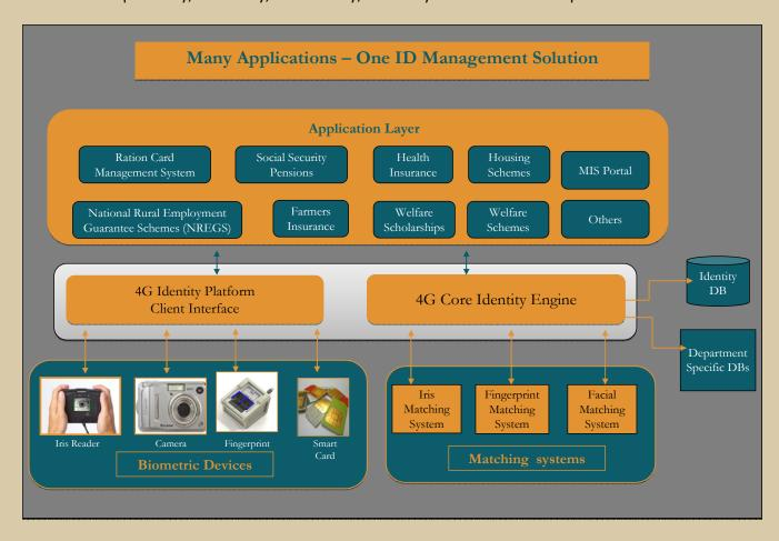
**Interoperability:** 4G's Identity Platform is capable of integrating not only multiple biometric devices but also search engine algorithms for iris, finger, face and biographic data.
