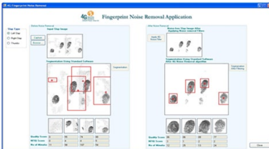
Fingerprint scanned with Noise, ghost images and also improper calibration of the device
